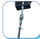
PARKING BRAKE ADJUSTMENT MECHANISM
