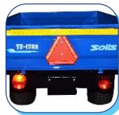
REAR REFLECTORS AND BRAKE LIGHTS FOR ENHANCED ROAD SAFETY
