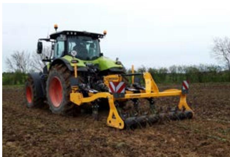
Cultiplow Platinum HD 3 m - 4 lame Sicurezza bullone - rullo Combimulch Steel-Pack
